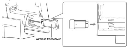
2 Insert a wireless transceiver into the subwoofer.
